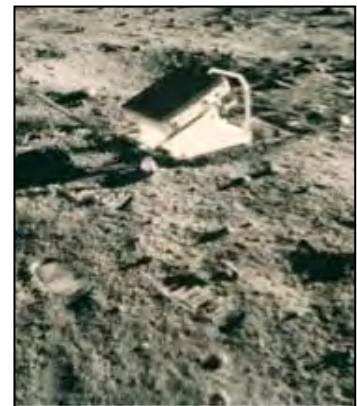
Fig. 3. Retroreflector placed on the Moon by the Apollo astronauts.
