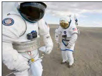
Fig. 2. Astronauts field test next-generation extravehicular activity (EVA) spacesuits on analogue lunar surface terrain at PISCES atop the Mauna Kea volcano on the Big Island of Hawaii.
